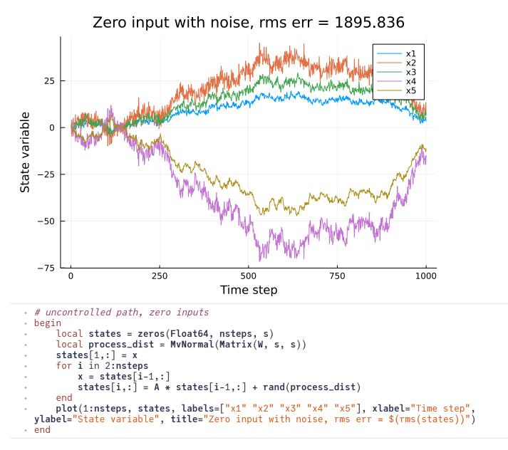
Next, we drive the system with random inputs, and this leads to it going off even further, because I didn't control the action of B the same way I did A. (I'm not really sure how to ensure the stability of a dynamic system defined by a non-square matrix, as there's no concept of an eigenvalue - this would be intellectually interesting to look at but doesn't really matter.)
